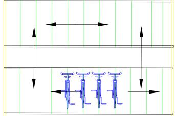
The VPSystem can be moved in the vertical position both to the right/ left and also to the front/back horizontally, so that the bicycles pushed together require a distance of approx. 300 mm.
